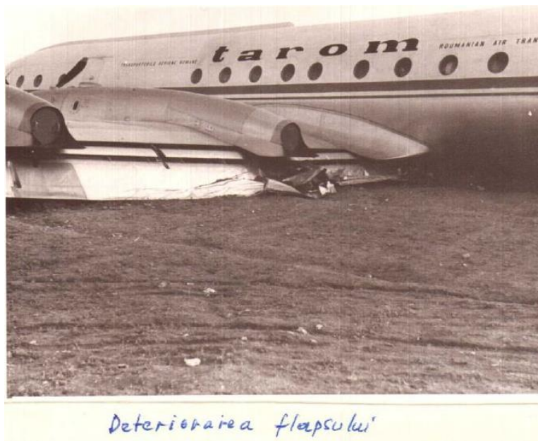
Fig. 6. The IL-18 airliner at the place of the forced landing. The flap was damaged.
