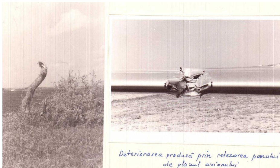
Fig. 7. The wing of IL-18 airliner clipped a tree during the forced landing.
